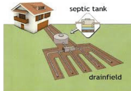
Typical residential conventional septic system showing septic tank, distribution box and drainfield.
